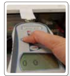
Figure 3 Ensure that the test strip and force guage line up horizontally
